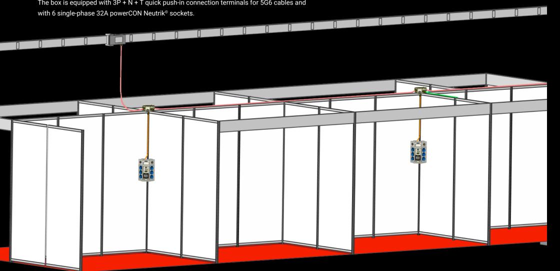
Thanks to the electronic power limitation of the COMPACT terminals, a single power supply connection can efficiently connect up to 18 power distributors, depending on the programmed power and the number of chained splitters:
